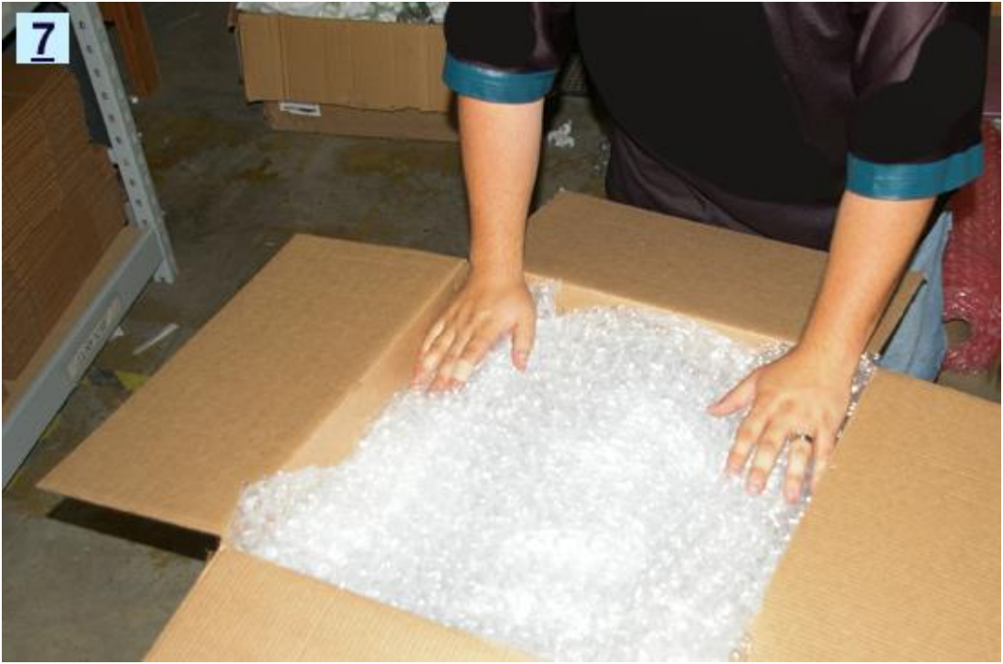
Use additional bubble wrap to ensure that there is no movement inside the box. Additional wads of bubble wrap into the corners of the box will help ensure a snug fit.
